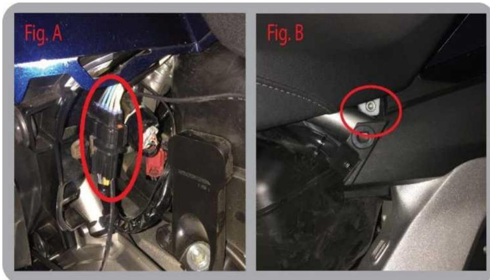
14. Remove the circled screw and feed the connectors through the indicated hole on your left side trunk hinge as shown in Fig. 10. These need to end up under the seat.
