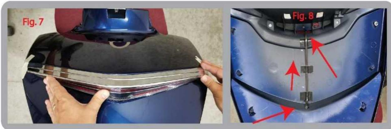
10. Route the wire straight up the inner lid of the tour pack and through the factory rectangular hole at the top. Use tape to hold the wire in place. (Fig. 8)
