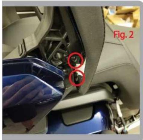
3. Remove the backrest to expose the trunk hinge screws. (Note there is a connector that must be unplugged by simply depressing the tab on the top)
