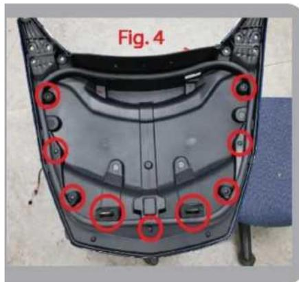
5. Remove the lid of your trunk and set it somewhere that it will not be damaged. Remove all inner liner and latch screws. Note where the long versus short screws are located. (Fig. 4)
