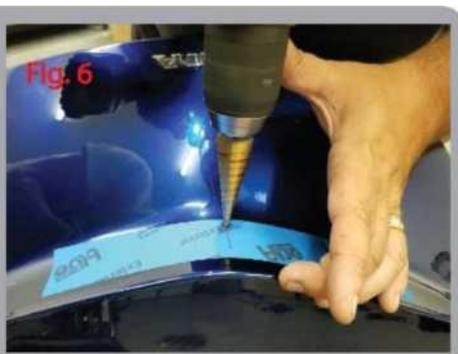
7. Drill a 9/16" hole where you marked the trunk lid, large enough to feed the connectors through. A step ' drill works well for this. (Fig. 6)
