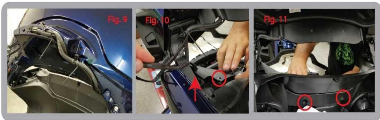
13. Open the saddlebags and remove the two side panels below the seat. Unplug the heated seat harness (Fig. A).
