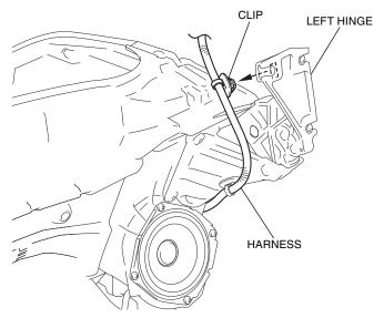
3. Remove the hinge rubber as shown.
