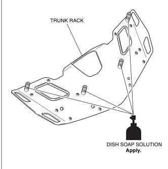
36. Install the trunk rack as shown.
