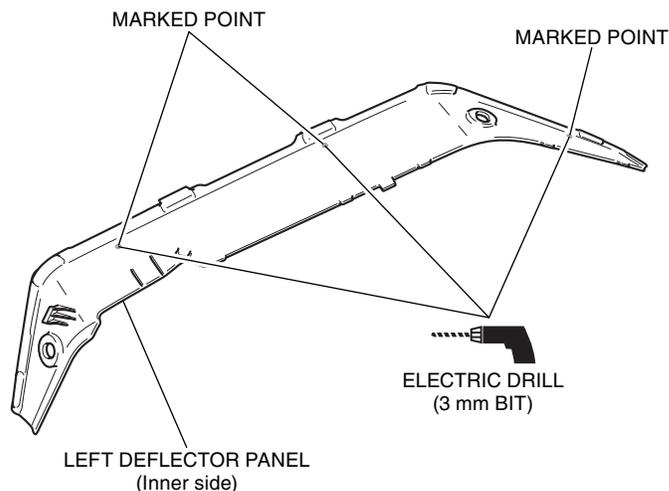
3. Drill at the marked lines of the left deflector panel as shown.
