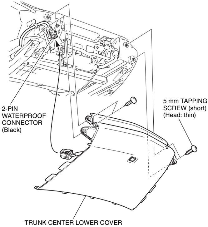
43. Remove the dummy connector as shown.
