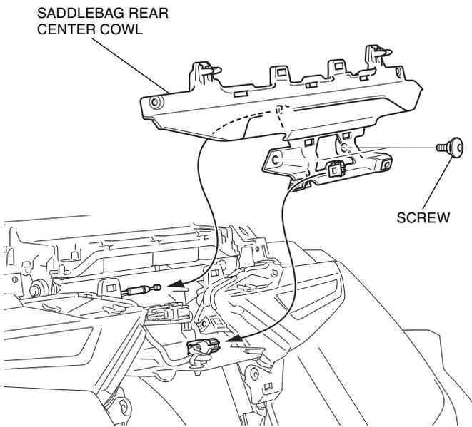
15. Remove the parts as shown.
