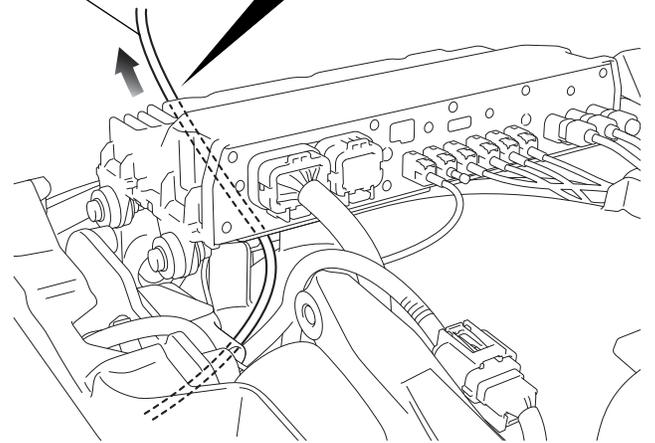
22. Remove the radio antenna as shown.
