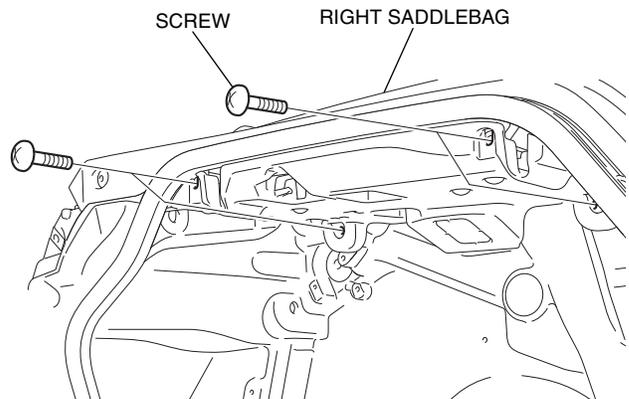
19. Move the right saddlebag catch and remove the plug as shown.
