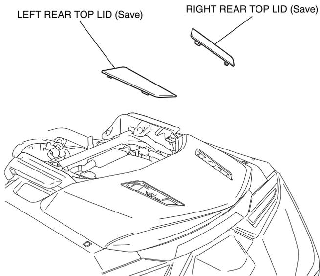
8. Remove the parts as shown.
