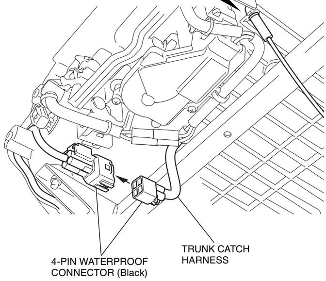
41. Install the trunk open switch as shown.
