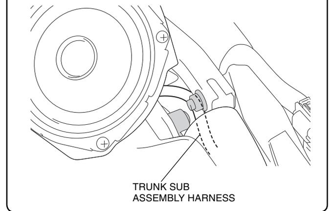
45. Remove the dummy connector as shown.
