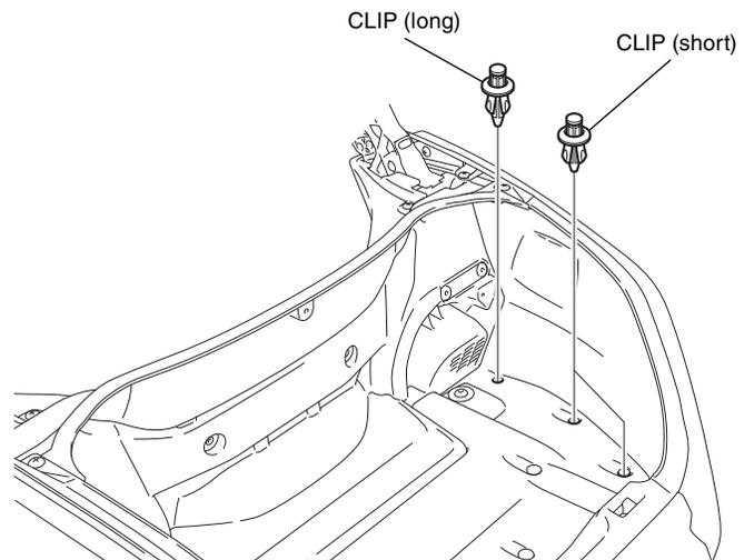
50. Install the trunk front lower panel as shown.
