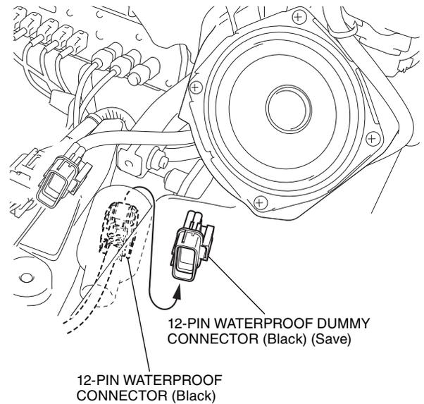
46. Connect the connector as shown.
