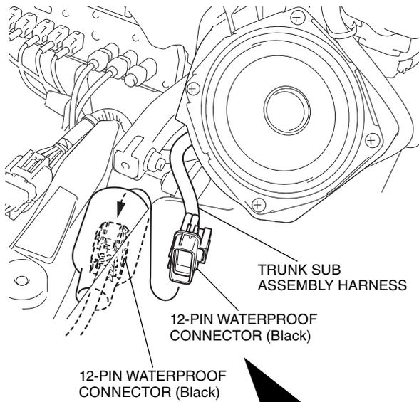
Route the trunk sub assembly harness as shown.
