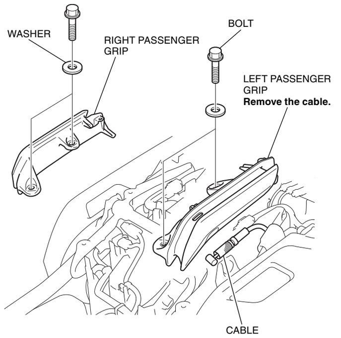
13. Remove the rear fender as shown.
