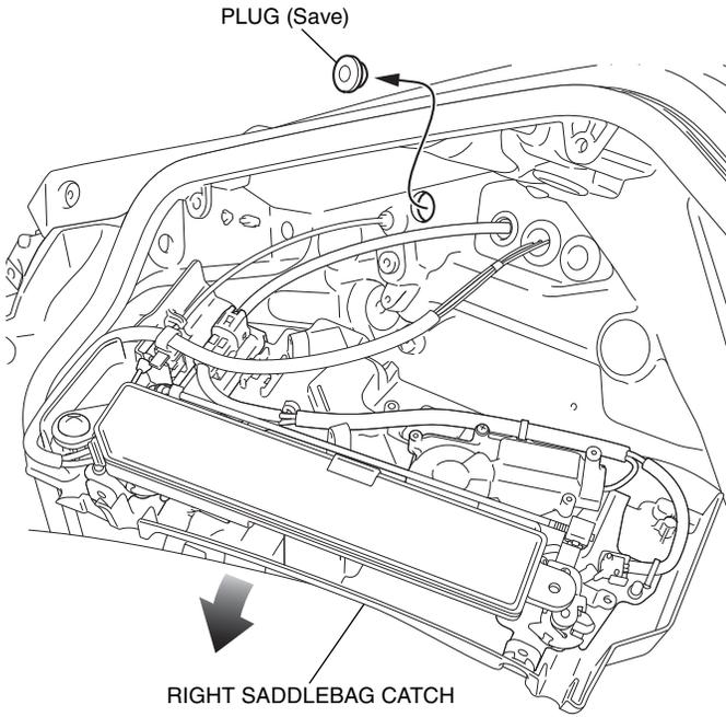
20. Install the emergency trunk cable as shown.
