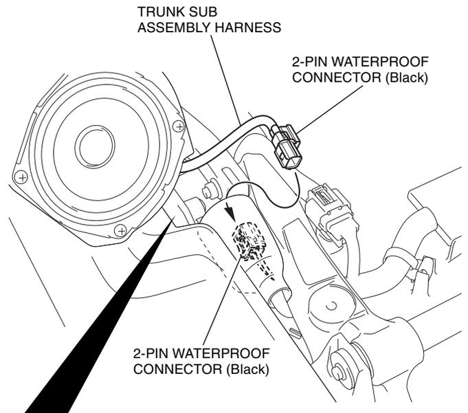
Route the trunk sub assembly harness as shown.
