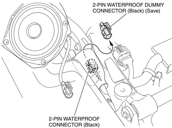
44. Connect the connector as shown.
