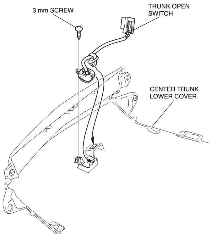
42. Connect the 2P black connector and install the trunk center lower cover as shown.
