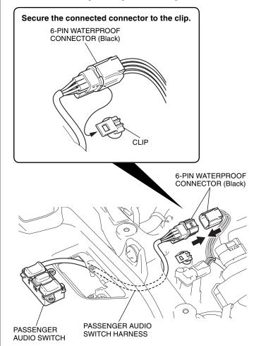
9. Install the passenger audio switch and right switch cover onto the right saddlebag as shown.
