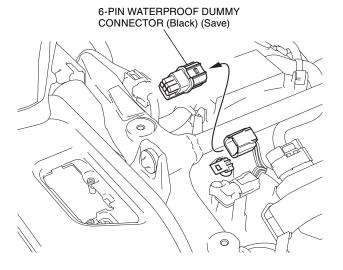
8. Route and connect the passenger audio switch harness through the right saddlebag as shown.
