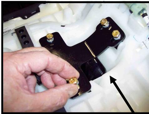
**Step 4:** Slide Mounting Bracket into slit in seat. Will have to push hard.
