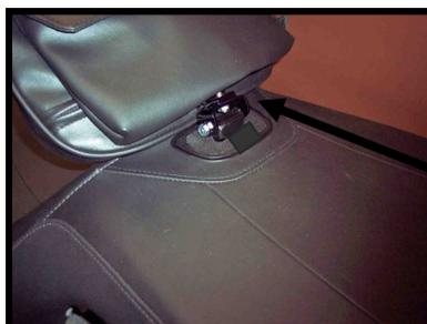
**Finally:** Install backrest to tube with bolt provided. Install seat on cycle, adjust backrest for comfort, and "Take a Ride!"
