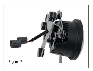
STEP 3. Install left light using three M6 x 50mm screws, flat washers, a 16mm spacer for the top and the side screws, one 20mm spacer on the bottom screw.
