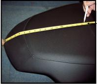
Step 3: Measure from Rear of seat forward 16 3/4".Mark center side to side.
