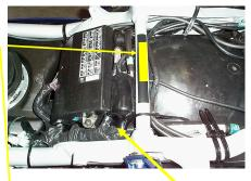
Note: Tuck all wiring in area, down between cross frame and black wiring junction box, to assure no wire gets pinched. Pull Velcro on T-Bar apart, peel off backing and stick in center of frame. (where highlighted in yellow). This protects cross frame and adds to rigidity of backrest.
