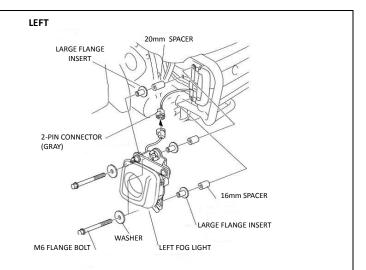
Note: There are six 2mm spacers in this kit. These extra spacers are for fine adjustment of your driving/fog light as needed.
