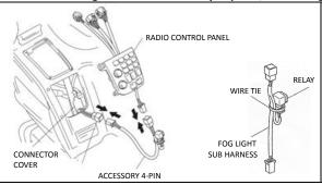
STEP 21. Place the relay and driving/fog light sub harness in the gap as shown.
