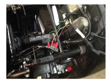
Picture shows area to remove wire tape. Use extreme caution when using sharp cutting tools to prevent wire damage.
