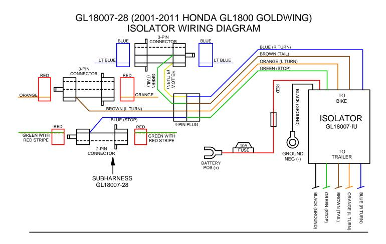
GL18007-28 (2001-2011 HONDA GL1800 GOLDWING) WITH 5-TO-4 WIRE CONVERTER & ISOLATOR
