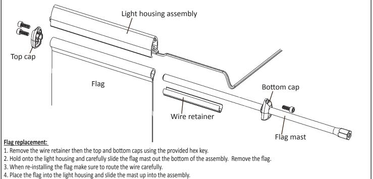
5. Attach the bottom cap first followed by the top cap. Reinstall the wire retainer.
