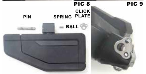
**STEP 6** On the front side of the adapter of the provided floorboard, insert the spring into the top hole, followed by the steel ball and click plate. When the floorboard is aligned with the motorcycle the flat edge of the click plate should facing towards the bike, and the steel ball should be covered by the bottom small hole of the plate.
