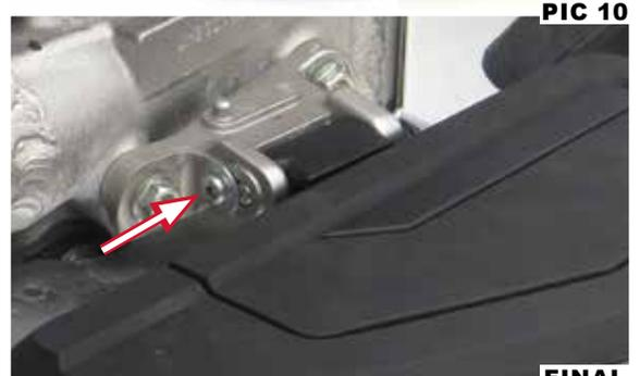
**STEP 9** Refer to PIC 10. Align the mounting holes of the adapter of the floorboard and pillion step holder. Insert the pillion pin from the rear of the holder, pushing it towards the front of the motorcycle. Test fold the step up and down to assure the pillion click plate is properly intact and the floorboard functions accordingly. The floorboard should stay in place when folded up.
