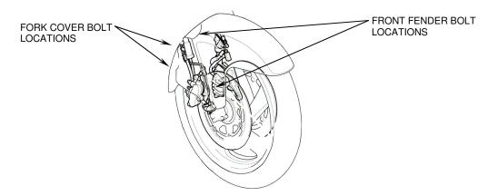
Figure 1 -REMOVAL OF FENDER AND FORK COVERS
