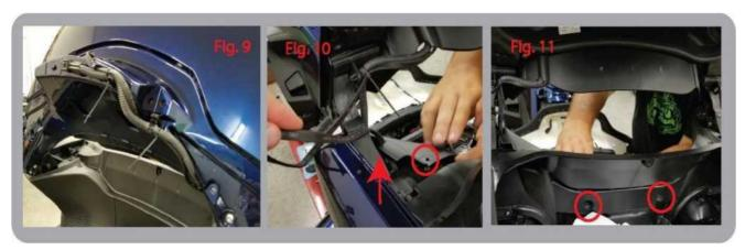
13. Open the saddlebags and remove the two side panels below the seat. Unplug the heated seat harness (Fig. A).
