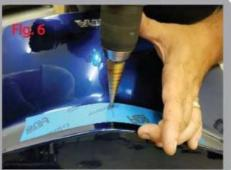
7. Drill a 9/16" hole where you marked the trunk lid, large enough to feed the connectors through. A step ' drill works well for this. (Fig. 6) G0048004, REV. - A
