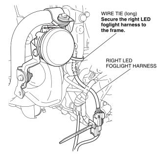
61. Secure the connector with the holder clip as shown.
