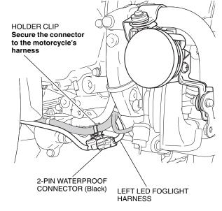
66. Secure the sub harness with the wire tie as shown. <GL1800BD/D/DA>
