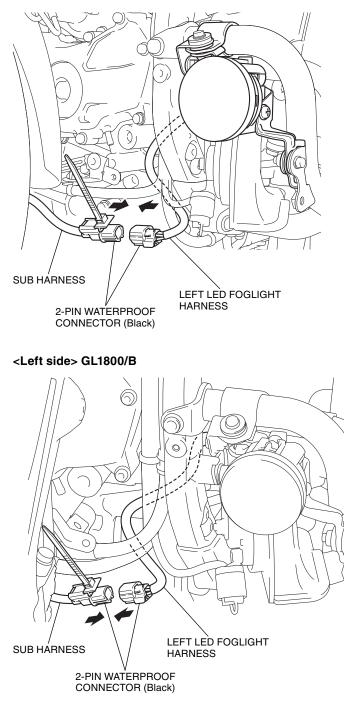
64. Secure the left LED foglight harness with the wire ties as shown.
