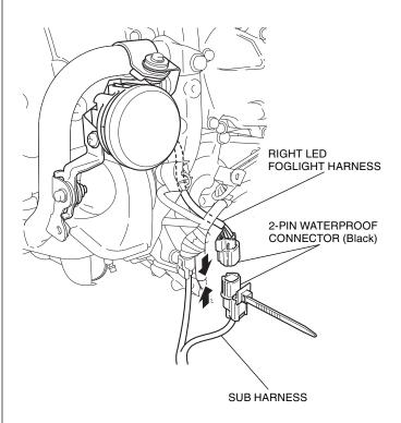
60. Secure the right LED foglight harness with the wire tie as shown.
