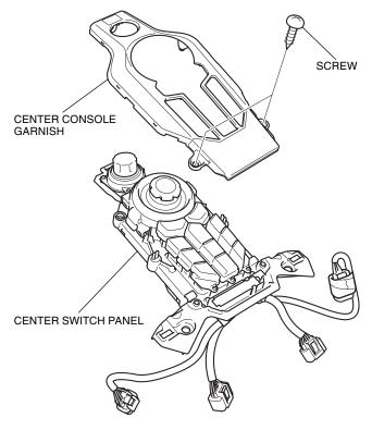
35. Remove the dummy switch as shown.
