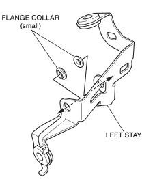
45. Loosely install the assembled left stay to the assembled LED foglight as shown.
