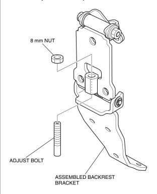
10. Install the special nuts as shown.
