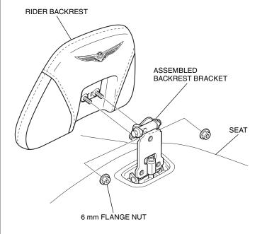
17. Tighten the loosely installed 6 mm flange nuts securely.
