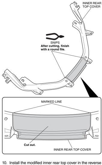
10. Install the modified inner rear top cover in the reverse order of removal.
