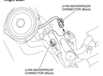
37. Install the dummy connector as shown.
