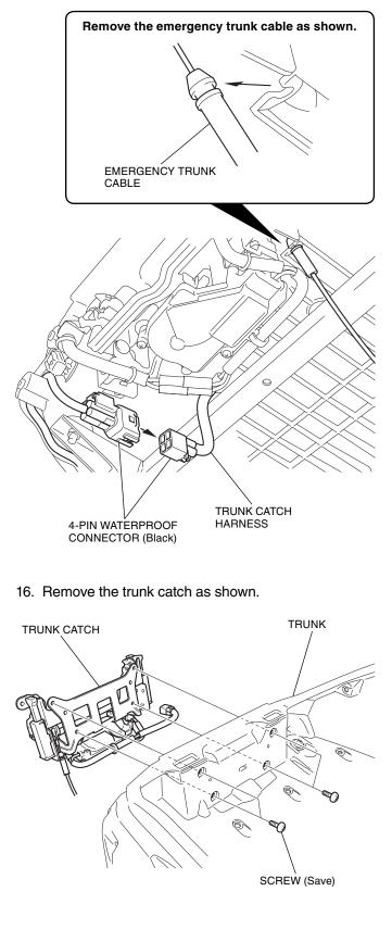
17. Remove the emergency trunk cable from the trunk catch as shown.
