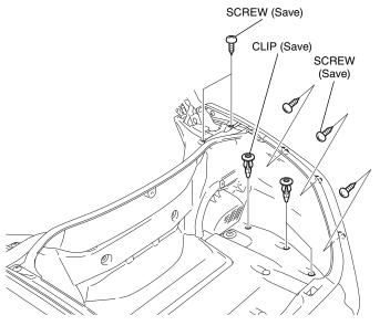
13. Remove the trunk right side cover as shown.
