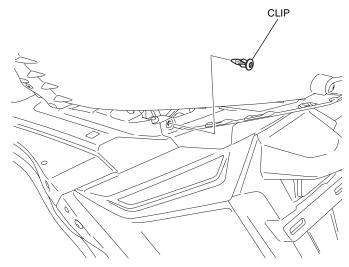
19. Remove the rear fender as shown.
