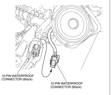
35. Install the dummy connector as shown.
