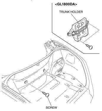
11. Remove the trunk front lower panel as shown.
