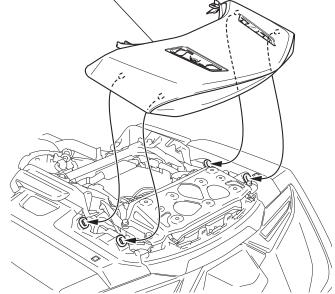
47. Install the clips and 5 mm screws as shown.
