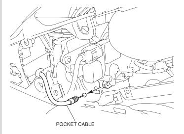
21. Remove the parts as shown.
