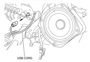
14. Disconnect the connector as shown.
