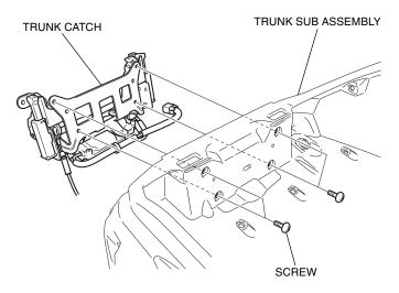
18. Remove the emergency trunk cable as shown.
